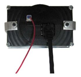
3. Connect the CAT5 cable to the clock. Route this cable back to the VHX control box.
