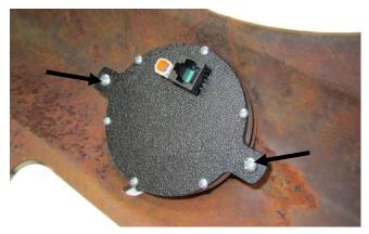
3. Connect the CAT5 cable and switch harness to the clock and carefully route these back to the VHX control box and refer to the Operating Manual to complete the VHX clock setup.
