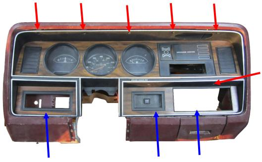
2. Remove and retain the (5) screws in the locations below to remove the stock gauges. Keep these screws separate from the screws retained in the previous step to avoid any confusion.
