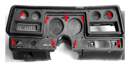
2. Remove the stock gauge cluster from the bezel. The gauge cluster is held in place by four screws in the center of the bezel, and two more along the top edge. Save the screws obtained as they will be re-used to secure the new VHX system.
