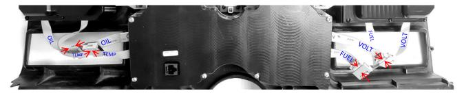
7. Connect the provided 36" CAT5E cable to the back of the VHX cluster as it is installed in the dash. Take care when routing the other end of this cable back to the control box mounting location.
