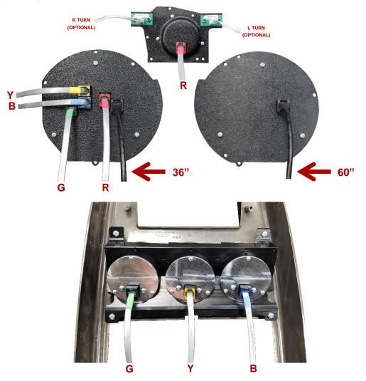
6. Carefully route the open CAT5e Cable ends to the control box mounting location. Refer to the main VHX manual for wiring instructions to complete the installation.
