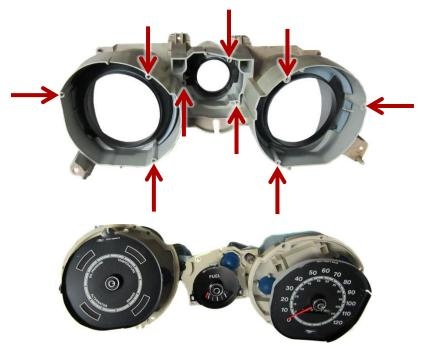
3. Mount the VHX displays into the original housings using hardware retained from the previous steps.
