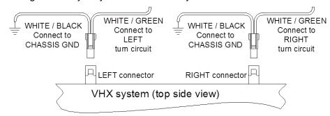
Connect the four provided Auxiliary Gauge Harnesses as shown below, matching color to color between gauge pods. Also connect the 36" and 60" CAT5e Cables to the speed and tach gauges respectively.
