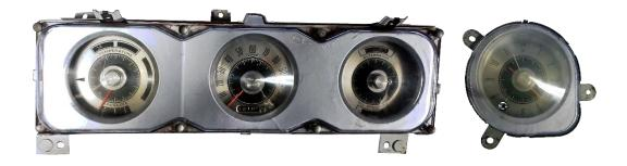
2. Remove all factory gauges, lights, circuits and fasteners from the original instrument housing. Make sure to retain the push pins that secured the original lens and faceplate. All other removed parts may be set aside, as these components will not be used with the VHX system.
