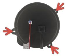
7. Mount the VHX system to the dash using the retained factory hardware from step one. Reinstall the dash pad.
