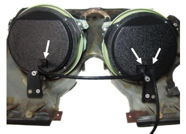
5. Peel the paper off the two block-off lenses needed for the back of the housing appropriate for your vehicle. Place them shiny side down in the two indicator openings. Use silicone to hold them in place and avoid handling until the silicone has cured.
