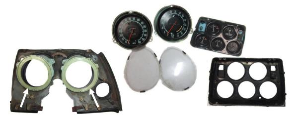
3A. The Speedometer and Tachometer are interchangeable side to side. Choose the orientation you prefer, then place the Speed and Tach on the main lens spacers and secure the gauges with the six (6) stock mounting screws. Use two (2) stock mounting screws to attach the ABS plastic brackets to the bezel and thumb screws to secure the brackets to the VHX gauges.
