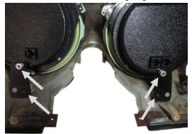
3B. Dashes with the vent by the driver's right knee will use the extended ABS bracket for proper Mounting.
