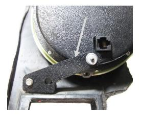
4. Once the VHX gauges are secured to the bezel; connect the 12" CAT5 cable to the Tachometer, and the other end to either port on the Speedometer, connecting the two halves. With the 36" CAT5 cable, connect one end to the open port on the Speedometer, and as the assembled cluster is installed into the dash, carefully route the other end of the cable to the control box mounting location.
