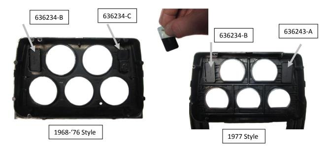
6. With the block-off lens in place, place the VHX center gauges over the back of the center bezel and secure the system by using the four (4) stock mounting screws.
