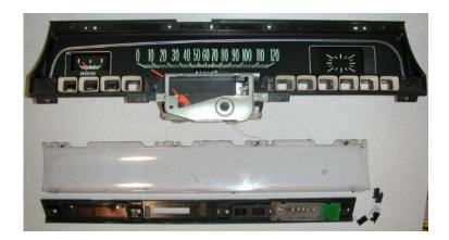
Remove indicator light panel to expose lens attachment. You will need to carefully cut or grind off melted studs to remove the lens. Remove gauges from back of cluster.
