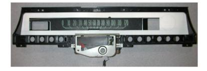
Using provided template mark area to be cut out of original speedometer display area. A silver marker works well for this. There is an area of the template that will need to be removed if you have the optional clock/temperature gauge.
