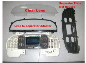
adapter and separator plate from the gauge cluster. You will not reuse the separator plate.
