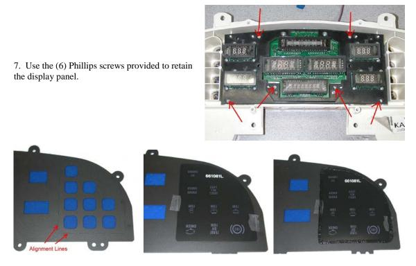
8. Set the new lens face down and use the lines etched in the back of the lens to line up the indicator light panels. Use tape to position them before applying a light bead of silicone around the edge to secure them.
