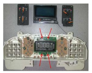
3. Remove outer gauges and the gear indicator/speed display cover.
