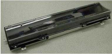
Place the clear lens and adapter plate on top of the Dakota Digital lens and use the provided screws to assemble.
