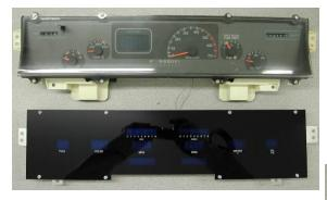
After removing the stock cluster from the vehicle remove the clear lens and black angled adapter plate.
