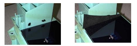
9. Place the original clear lens over the system lens. The notches on the top of the systems lens will align and position it. Use the original screws to hold the lens on place. Allow the silicone to dry before installing the cluster.
