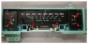
3. Remove the three screws pointed to in the photo at right.
