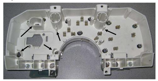
With the light bulbs and electrical contacts removed, use a die grinder or cutoff wheel to remove the plastic bosses from the stock housing as illustrated by the arrows in the photo above.
