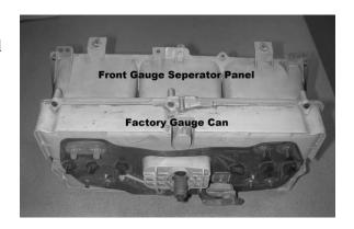
• Using the supplied templates, mark the outer openings on the gauge separator panel for material removal as shown. This is the minimum that needs to be removed. If you remove more material it is recommended to leave about an 1/8" ledge for the lens to sit on and be glued to.
