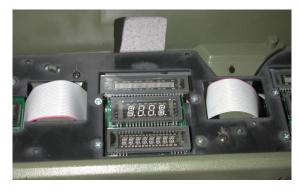
Place gauge subpanel display assembly into the dash.
