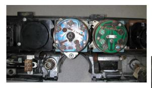
Install included #8-32 X  $\frac{1}{2}$ " hex standoffs on original gauge mounting studs, hand tightening as far as possible. Up to  $\frac{1}{16}$ " gap between standoff and hex of the original stud is acceptable. Be careful not to over tighten causing damage to the plastic risers.
