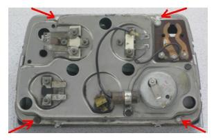
6. Remove the center gauge cluster from the vehicle. From the back side, remove the four screws as indicated by the arrows in the photo at left which hold the stock gauges to the bezel. The stock gauge assembly can be set aside.
