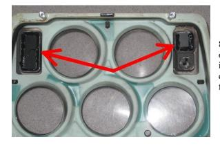
8. Included are some lenses that can be used as block offs for the openings at the sides of the top two gauges as indicated by the arrows in the photo at left. Due to factory changes over the years, three different sizes are provided. The small one is not square and will only fit in one direction. Set these in place and secure with silicone.
