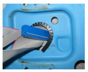
3. Use the provided flexible grommet material on the edge of the mechanical cable openings on the original gauge cans to protect the ribbon cables. A few dabs of silicone will help hold it in place. Pass the ribbon cables through the lined cable openings until the gauge assemblies sit into the cans and the cables are not being pinched.
