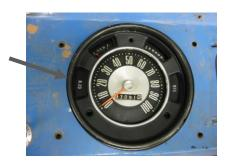
2. Remove the cluster from the bezel so you are left with a bare bezel.
