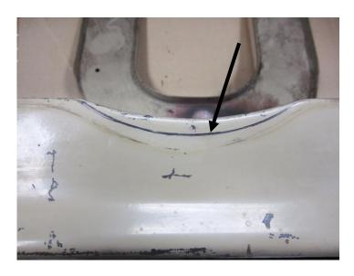
4b. Carefully remove the area of the dash that interferes with the VFD3 system fitment. Test fit and make additional cuts as needed until there is no contact between the VFD3 system and the dash.
