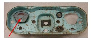
3. Remove the screw from the front of the battery indicator light on the top left as indicated by the arrow in the photo at left.
