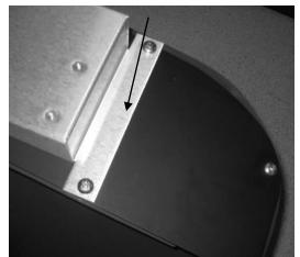
Place screws through the can into the lens and through the bezel. Then start a lock washer and nut on the bottom.
