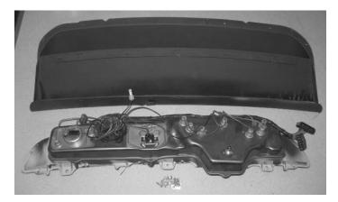
Below are the pieces you will use to install the Dakota Digital gauge package. The system is mounted in an aluminum can that has mounting tabs in proper locations that will allow you to bolt the system and lens to the original bezel with the supplied #10-32 mounting hardware.
