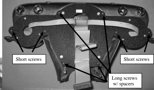
Once all hardware is started, tighten it up to complete the installation of the system.
