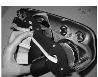
The system is mounted in the stock housing with the supplied #8-32 mounting hardware. Four shorter screws go towards the edges and four longer screws with nylon spacers in center section. (photos on next page)
