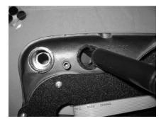
Reinstall the cluster in the dash, routing the ribbon cable from the displays to the control box. Make sure the ribbon cable isn't pinched or crimped by other dash components once the cluster is fully installed.
