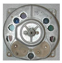
Before disassembly, mark the 12 O'clock position on the bezel for lens alignment.
