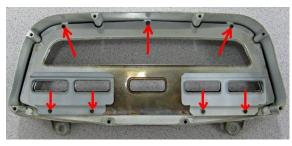
3. Remove the 7 screws, as indicated with arrows in the photo at left, which hold the gauge separator plate and glass lens into the bezel. The screws will be reused to hold the new colored lens in place. The separator plate and glass lens will not be and can be set aside.
