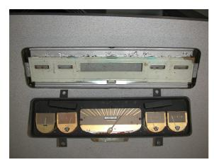
Using a small pliers or side cutters straighten the bent over crimps holding the housing halves together.
