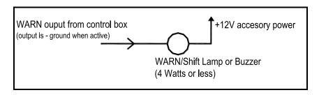
If you need the warn output to be "active high" or provide a +12V voltage to power something larger than 4 Watt, a standard 12V relay such as Dakota Digital RLY-1 can be used to accomplish this.
