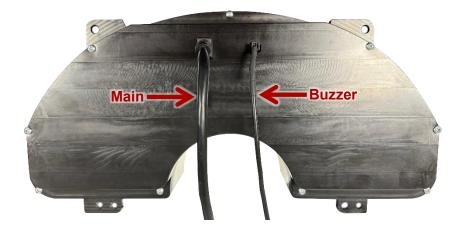
3. Mount the RTX display to the vehicle's dash using the four retained factory screws from step one.
