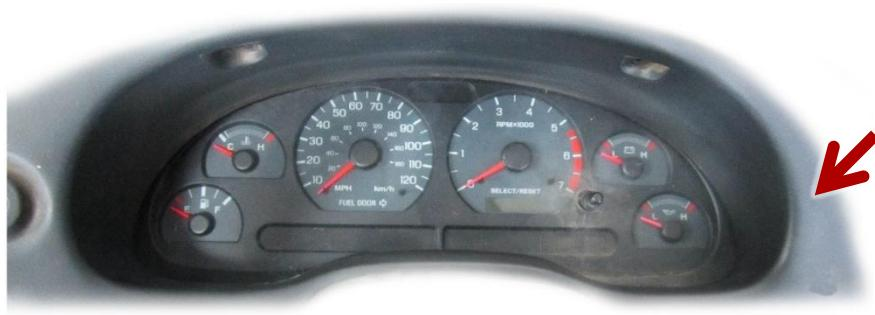
2. Remove the stock gauge cluster by removing the four screws holding the system to the dash structure; be sure to keep these screws as they will be reused. Now is a good time to clean the bezel and dash pads.
