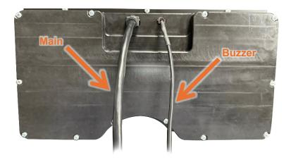
3. Mount the new RTX display to the dash using the four original screws retained during disassembly.
