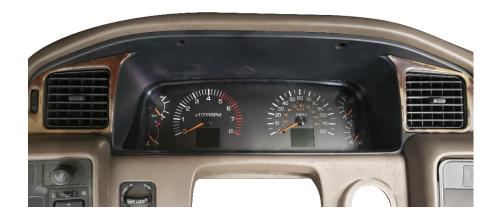
6. Stock 3-Wire alternators may need an additional wiring connection at the gauge cluster connector. This will 'excite' the alternator telling it to begin charging. This can be done using the included **Alternator Load Harness**.
