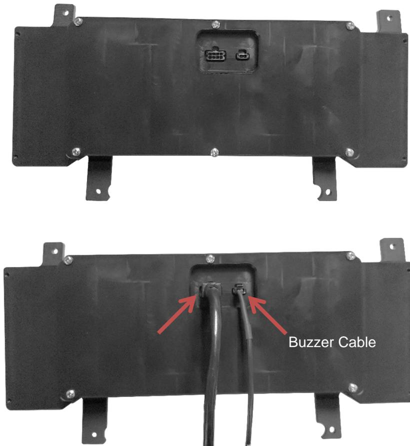
4. Install the RTX system into the dash. Align the four mounting holes and re-use the factory screws to fasten the RTX gauges into the dash.
