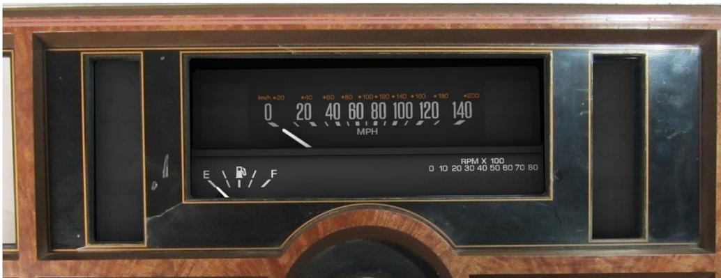
6. Stock charging systems will need an additional wiring connection at the gauge cluster connector. You will need to add a 300 to 500-ohm resistor between Pin 3 (Brown wire) and Pin 15 (Pink/Black wire). The provided alternator load harness can be used to achieve this.
