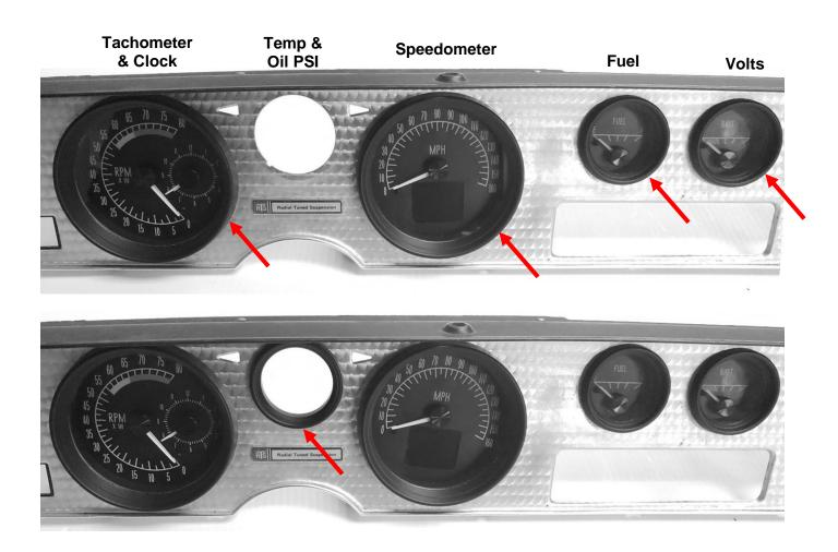
5. Flip the system over and fasten the trim ring to the bezel using the provided lock nut / rear half.
