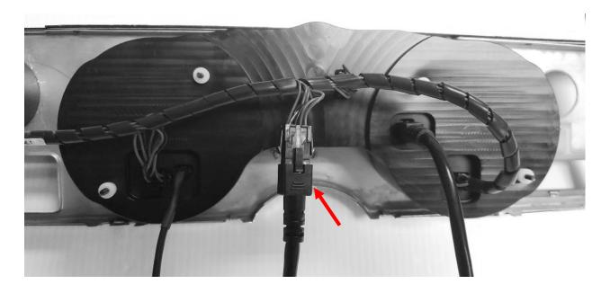
10. Carefully re-install the dash bezel with mounted RTX system into the car using factory hardware and refer to the main manual for wiring instructions to complete the RTX installation.
