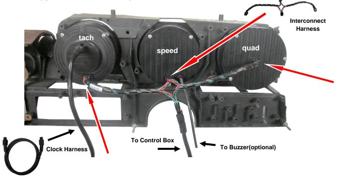
4. Re-install the gauge bezel to the dash housing using the factory hardware and refer to the main manual for wiring instructions to complete the RTX installation.
