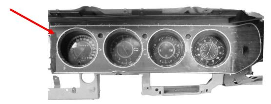
2. Remove the stock gauge cluster by removing the four (4) screws and retain the hardware for reassembly.
