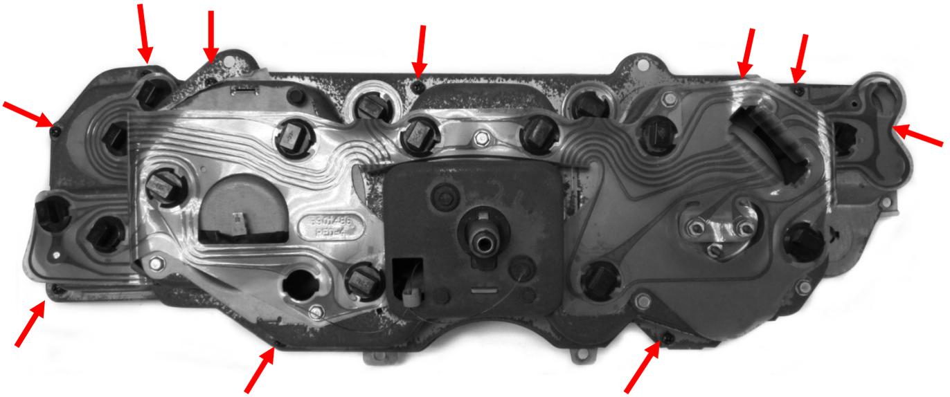
5. With the factory gauges and lenses removed, you will be left with a bare carrier, as shown below. Fit the ABS plastic headlight bracket over the back of the headlight switch opening and re-install the headlight switch
