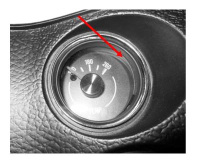
5b. The RTX system should align tightly and the lens should sit flush with the bezel. 6. Secure the bezel to the dash with the four original screws. Refer to the main manual for wiring instructions to complete the RTX installation.
