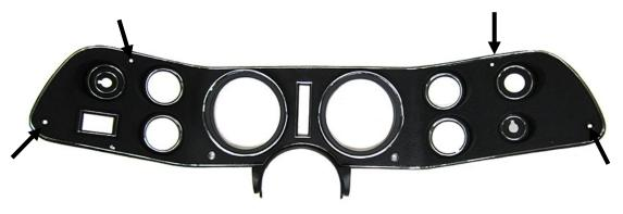
2. Remove the four screws holding the gauges into the dash. These screws will be re-used for the RTX gauge installation.
