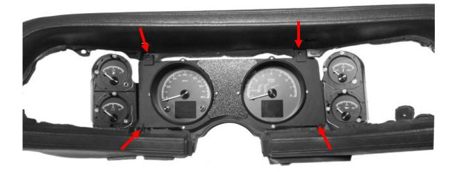
5a. Align the bezel over the gauges. Watch carefully so you don't scratch or damage the lens.
