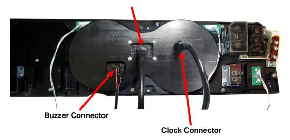
7. Re-install the gauge cluster to the dash using the factory hardware and refer to the main manual for wiring instructions to complete the RTX installation.
