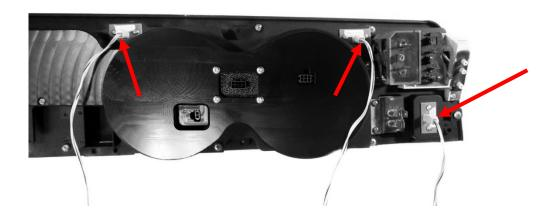
6. Connect the provided Main Harness, Clock Harness and Buzzer (optional for audio feedback) to the back of the RTX system.
