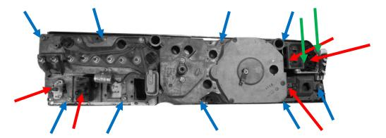
3. Mount the bezel to the RTX system by reusing eight of the nine screws that mounted the bezel to the factory cluster. The included 7/8" length screw will be the ninth screw and is located on the lower portion between the Speed and Tach, shown by the blue arrow.
