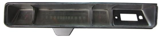
2. Remove the eight screws that mount the stock gauges to the bezel. Retain the stock hardware for reassembly. The stock gauges can be set aside; they will not be reused.
