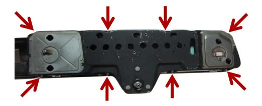
3. The stock clear lens is not needed but can be left in place if desired. To remove the clear lens, loosen the bottom four studs and the lens will slip out. Make sure to re-tighten the studs after removing the lens.
