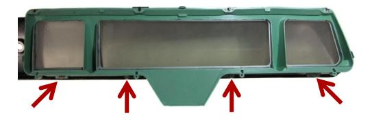
4. Mount the RTX system to the back of the bezel spacer using the stock hardware similarly to how the stock gauges were mounted. Note the longer screws are used for the top portion.
