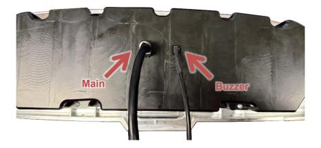
6. Re-install the gauge cluster to the dash using the retained factory hardware and refer to the main manual for wiring instructions to complete the RTX system installation.
