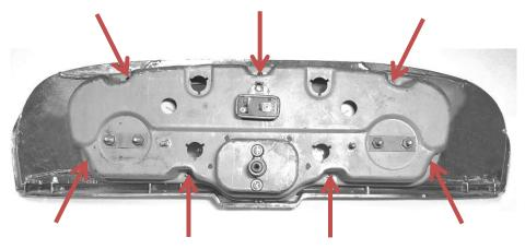
4. Carefully place the RTX display into the factory bezel and fasten using the retained original hardware. Make sure the aluminum spacer sits flush against the edge of the bezel.
