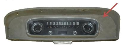
2. Remove the gauge housing from the front bezel by removing four screws on the bottom and three on top. Retain this hardware for reassembly. The bezel and related mounting screws will be the only items reused.
