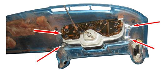
3. Remove the OEM bezel from the stock gauge by removing the eight (8) screws indicated below.
