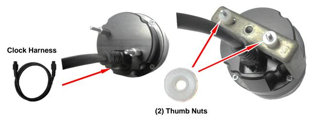
6. Mount the auxiliary gauges to the OEM bezel using the provided #6-32 short screws in the locations below. It is advised to use a magnetic screwdriver to line up the side screws.
