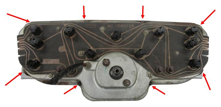
4. Completely strip the bezel of all remaining components, light guides, and indicator panels. If removing the factory gear indication, the provided blackout lens may be used. Peel the protective cover off the Blackout Lens and place it over the gear indicator opening with the shiny side facing out towards the driver and glue it in place using a black RTV silicone or similar to. Let the silicone fully setup and dry before moving on to the next step to prevent damage to the Blackout Lens.
