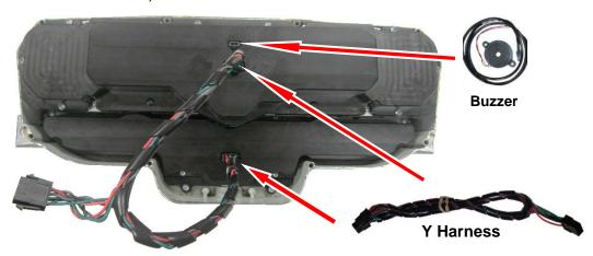
9. Connect the 36" main cable to the Y harness that is attached to the system. Connect the main cable and clock cable to mounted control box location
