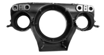
2. With the stock housing lying face down, install the RTX gauges into the housing using the supplied screws and lock washers. The Gas gauge mounts on the left and the Temp mounts on the right when looking at the system from the back.
