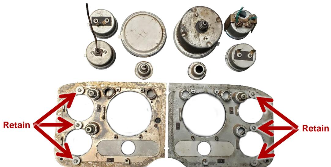
3. Insert the four smaller RTX displays into the outer openings from the back side. Fasten these displays down using the original screws with washers retained during the previous step.
