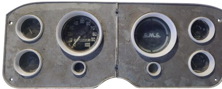
2. Remove the original gauges and fasteners from the factory dash panels. Do not remove the six screws with washers that retain the four outer gauges, as these will be reused when mounting the RTX displays.
