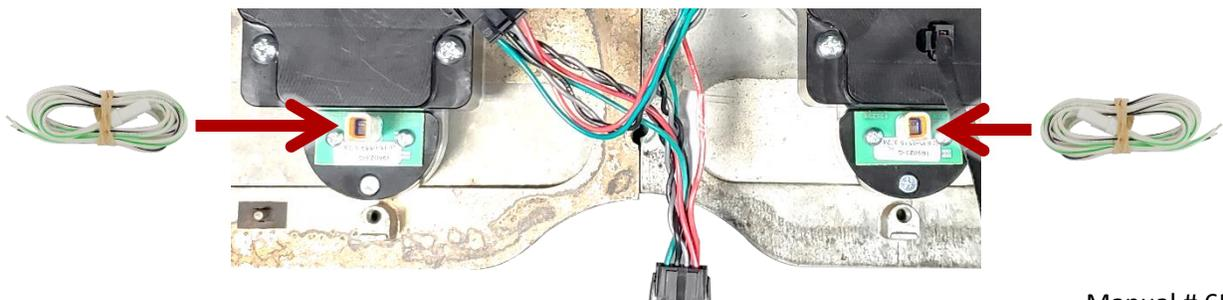
7. Re-install the assembled instrument panels into the dash. Refer to the main RTX manual for wiring instructions to complete the system installation.
