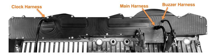
4. As the assembled cluster is installed into the dash, take care when routing these cables to the control box to avoid pinching. Re-install the cluster into the vehicle and refer to the main manual for wiring instructions to complete the RTX installation.
