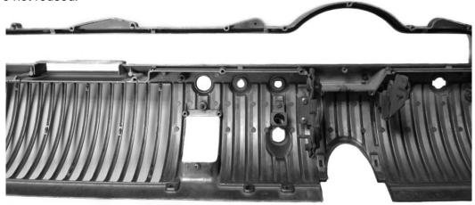
2. Remove the clear protective tape from the lens of the RTX system. With a Phillips screwdriver, carefully mount the Dakota Digital gauge cluster to the factory bezel. Use the supplied (12) #8-18 screws with lock washers as indicated by the *blue* arrows and the (4) #10-16 screws and lock washers shown by the *orange* arrows. Be sure the new RTX cluster fits the bezel with no gaps before tightening.
