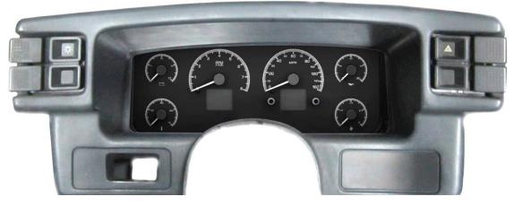
Stock Mustang charging systems will need an additional wiring connection at the gauge cluster connector. You will need to add a 300-to-500-ohm resistor between pin 14 (LG/R wire) and pin 2 (R/LG wire). The provided alternator load harness can be used to achieve this.
