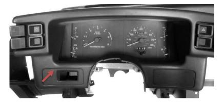
2. Remove the stock gauge cluster by removing the four screws holding the system to the dash structure. Be sure to keep these screws as they will also be reused. Now is a good time to clean the bezel and dash pads.
