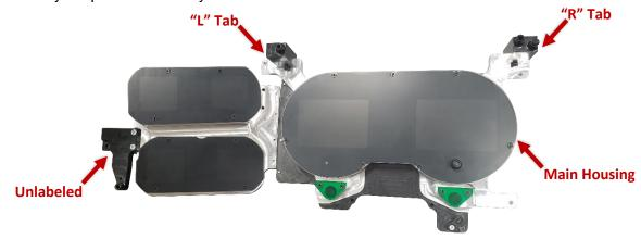
The remaining unlabeled tab goes on the bottom left side of the system, between the satellite gauges. Making sure the countersunk side of the tab is facing away from the rest of the unit, fasten this tab to the GRFX system with the two included **6-20 x** <sup>3</sup>/<sub>4</sub>" **Flat Head Screws**. This tab can be tightened until flush.
