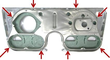
2. Remove the stock gauges, separator plate, and lens from the bezel. The only item to be reused is the original front bezel; the other pieces can be set aside. Now is a good time to clean the bezel and remove any dirt or old lens gasket material.
