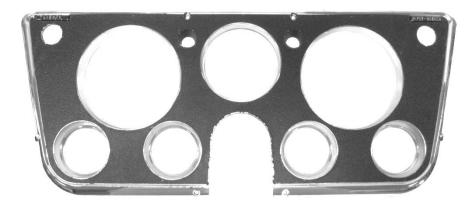
3. Secure the GRFX system to the bezel with the eight screws removed from the stock gauges.
