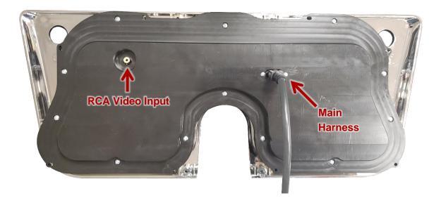
6. Re-install the gauge panel into the dash using factory hardware and refer to the Main GRFX Manual for wiring instructions to complete the installation.
