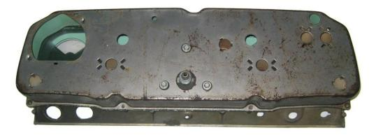
2. Remove all factory components from the original bezel. This will be the only item to be reused.
