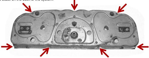
2. Remove all factory components from the original bezel. This will be the only item to be reused.
