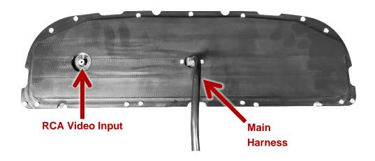
5. Re-install the instrument cluster into the dash and refer to the Main GRFX Manual for wiring instructions to complete the GRFX installation.
