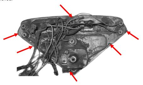
3. Next, cut the supplied foam into 1.5" long strips, and then cut the strips in half lengthwise so you have four pieces total. Install the foam blocks on top of the four bosses around the edge of the bezel to help prevent any lens rattles. The foam will compress against the lens once the system is installed.
