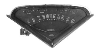
2. Remove the six screws holding the gauges to the bezel so the stock gauges, separator plate, and lens can be removed.
