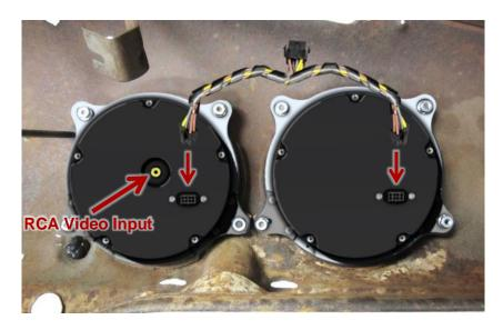
6. Connect the provided **36**" **Main Harness** to the open end of the interconnect harness.
