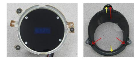
7. Position the new clear lens in place of the original using the two notches indicated with the yellow arrows for alignment. Use silicone in the areas indicated with the red arrows to retain the lens.
