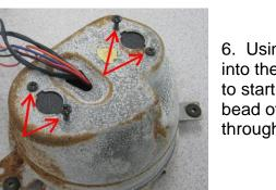
6. Using the 4 included screws provided secure the clock assembly into the housing using the light cover tab holes. It is recommended to start all 4 screws then tighten in a crisscross pattern. Place a bead of silicone around the edge of the opening that the wires pass through to keep them from chaffing.
