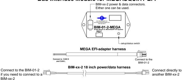
This Bus Interface Module is designed to read engine information from specific MEGASQUIRT EFI kits. These kits include: Megasquirt-2, Microsquirt, MSPNP2, Microsquirt-module based ECUs with firmware MS2/Extra 3.4.x or later, Megasquirt-3, MS3-Pro, MS3-Gold, MSPNP-Pro, MS3-Pro-module based ECUs with firmware MS3 1.4.x or later. The module is connected to the MEGA through the CAN-bus CAN H and CAN L on the MEGASQUIRT harness.
